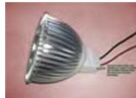
8. Connect the spotlight output wires to the input wires by soldering.
