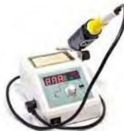
Some bases offer heat profiles features that allow changing the amount of heat of the tip for facilitating soldering of different components.
