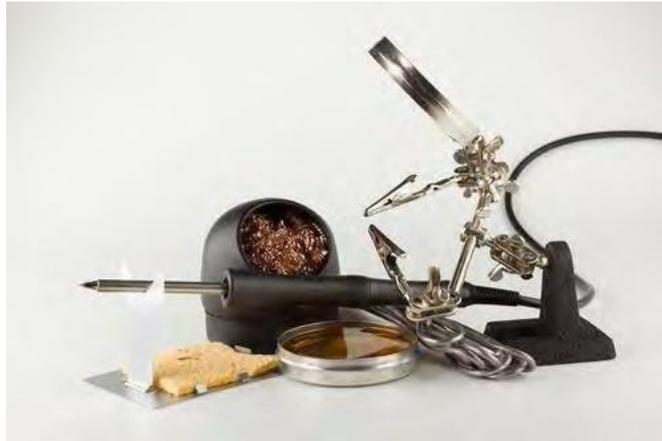
Basic parts of a soldering iron
