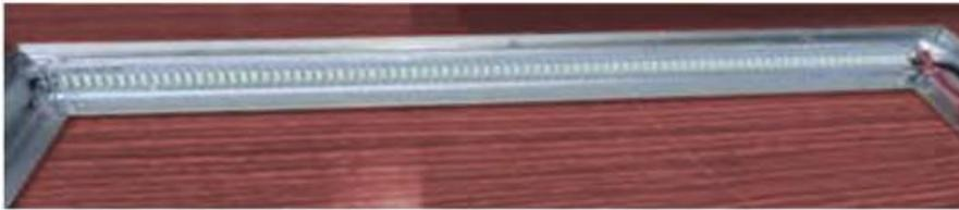
2. The extrusions are placed together to form a frame.
